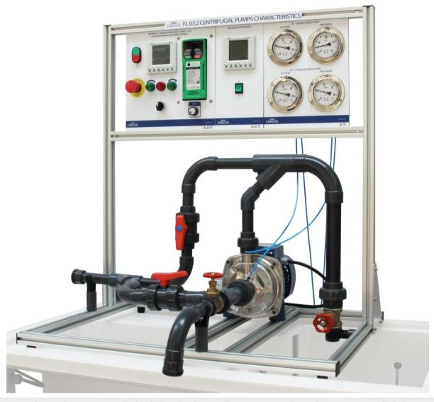
The equipment is designed to operate on hydraulic bench. The installation is mounted on a frame constructed of aluminum, with a system of pipes and valves that allow it to be coupled hydraulic pump and bank equipment in series or in parallel.
